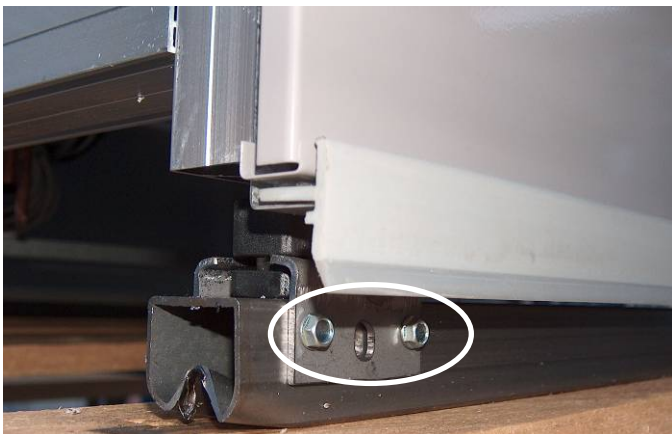
Fig. A1: detail of clip fastening screws
