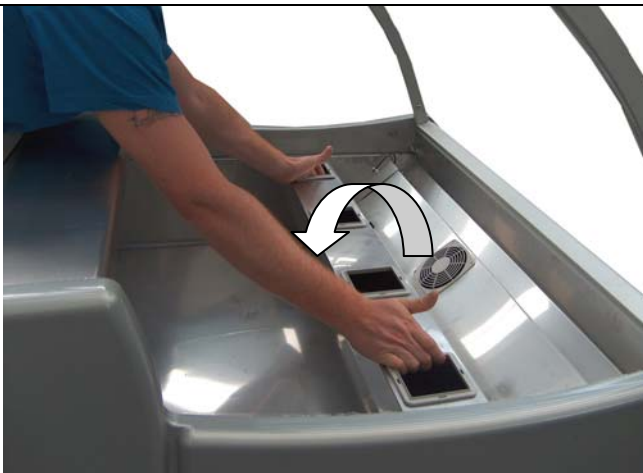
Fig. B: removal of evaporator cover
