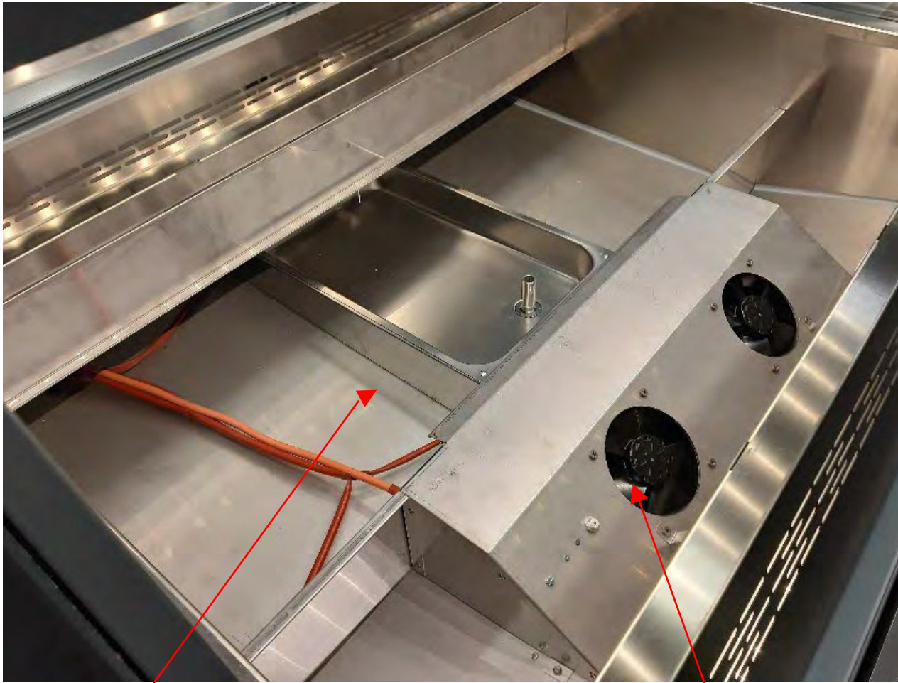
Heating element and fans placed inside the fan holder
